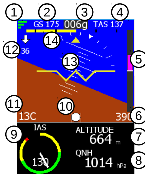
Figure 5: EMSIS primary flight display page.
