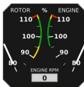
Figure 44: The combination of rotor RPM and engine RPM. Both scales are in percentages.
