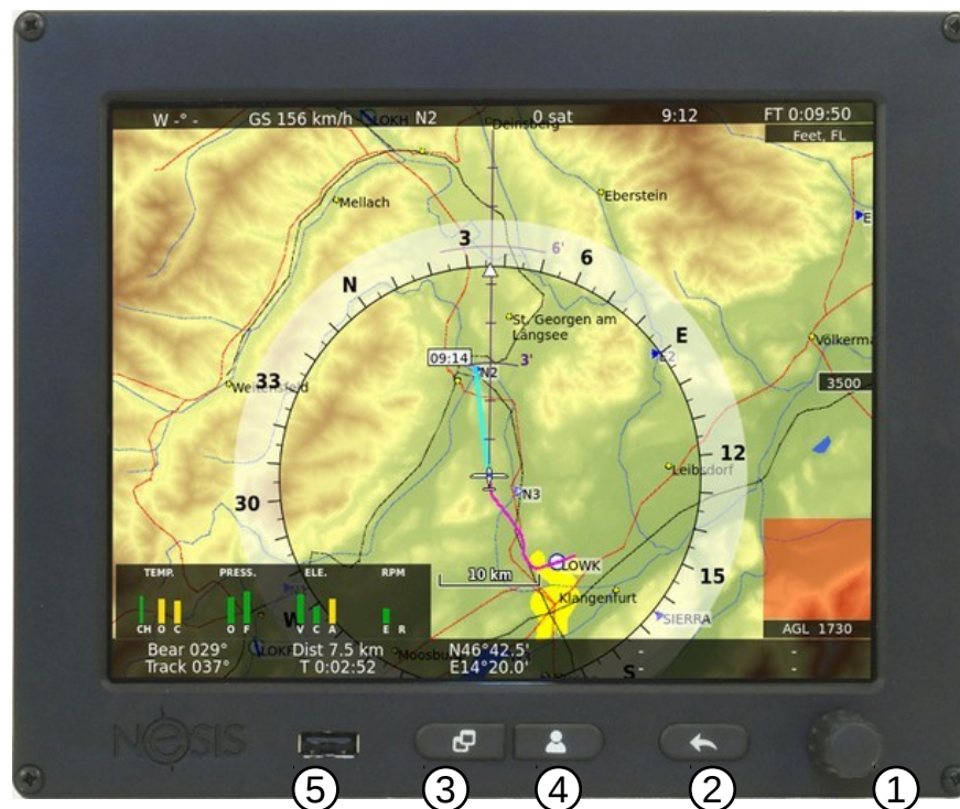
Figure 4: Organization of the NESIS front panel.
