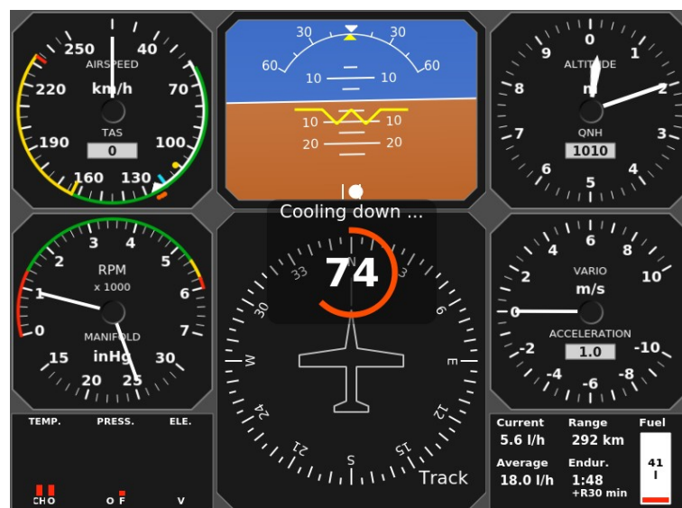
Figure 33: Cooling countdown is shown on the middle of the screen.
