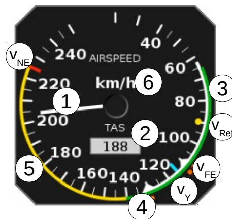
Figure 38: Airspeed indicator optimized for an aeroplane using two step landing flaps.
